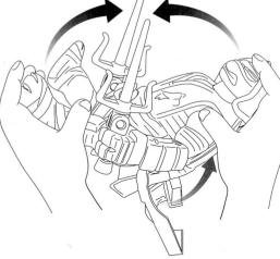
4. Pull the feet up towards the head (note the support bracket will also fold in) until it locks into place
