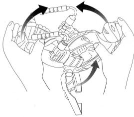
4. Pull the feet up towards the head (note the support bracket will also fold in) until it locks into place
